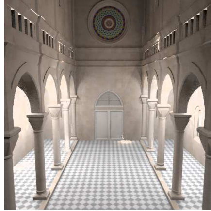
Figure 4: When the minimum distance test isn't used as was done for this image, there are unsightly bright spots around the points where the virtual light sources are on surfaces, due to the 1/r^2 term taking on a large value there.
